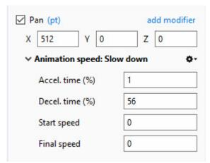
**Acceleration Time** and **Deceleration Time** can be set separately or together to produce the Speed Option effects of Version 8
